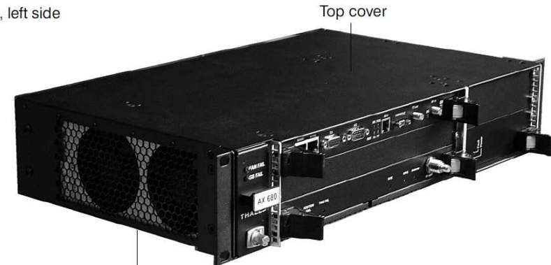
Air Inlet, Fan, dust filter
